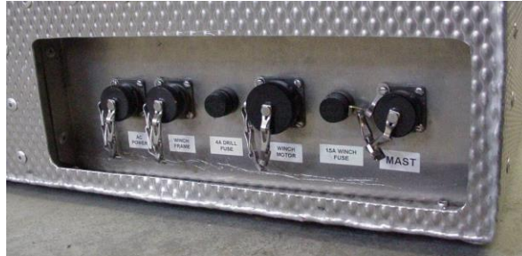
Figure 13 – Control Panel Back Panel
