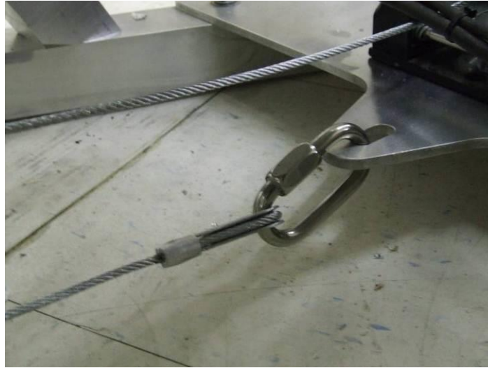
Figure 44 – Boom Winch Cable Termination
