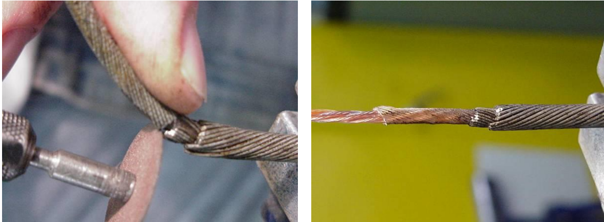
Figure 26 – Winch Cable Preparation
