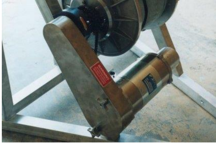
Figure 6 – Installing the Cover Plate
