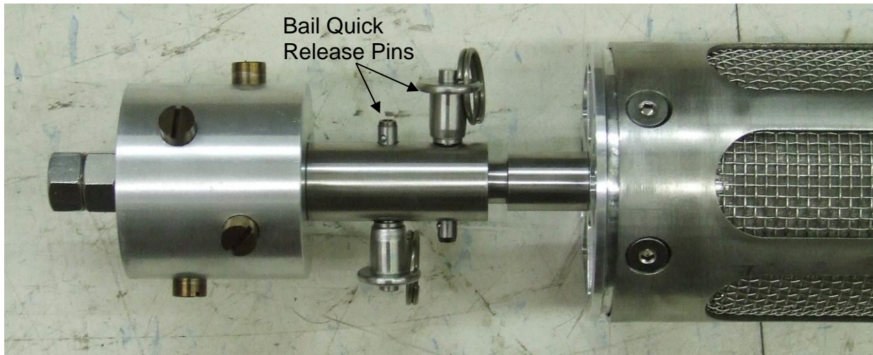
Figure 48 – Booster Pump Connection
